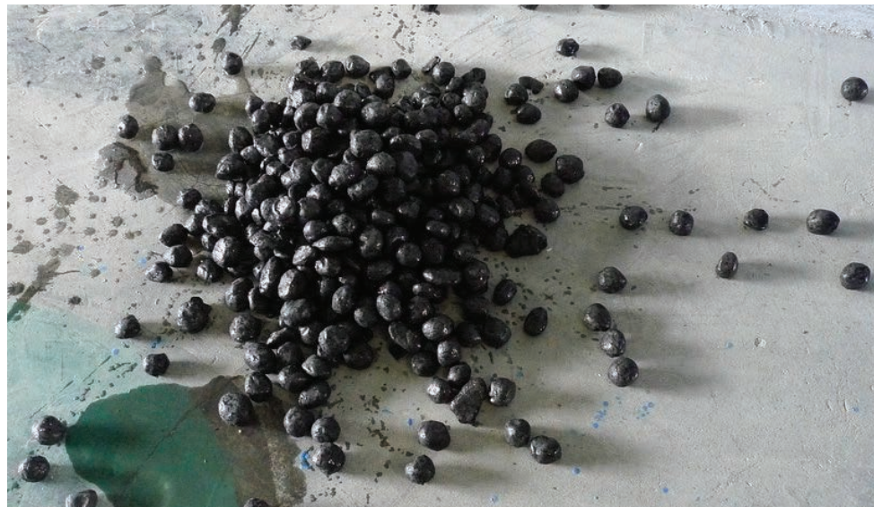
The image above shows pitch balls, which formed inside the screen before application of Busperse.
