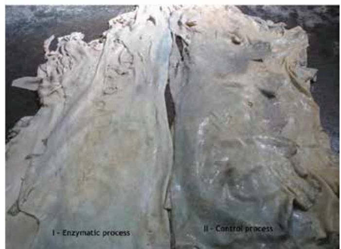
Figure 5. Photographs of limed pelts from enzymatic (I) and control (II) processes on pilot trials.
