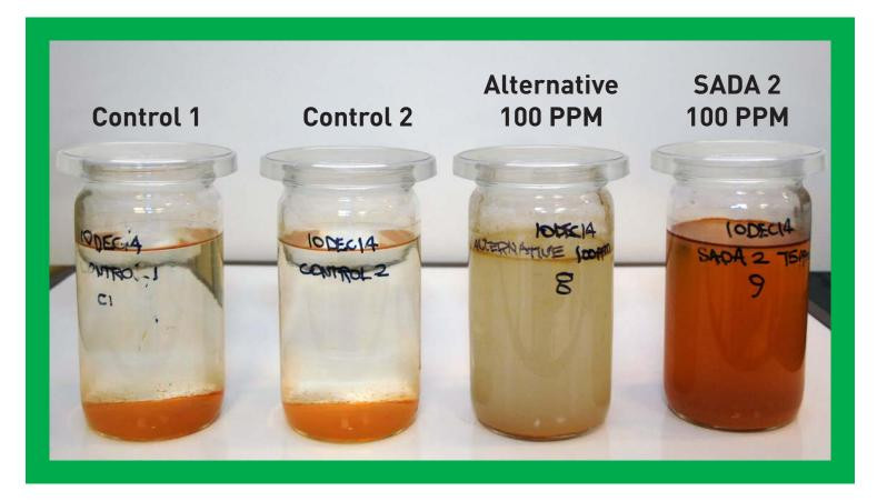
The corrosion test was done with steel pipe sections in synthetic water (300 ppm  $CaCO_3$ , 75 ppm  $MgSO_4$ ; pH 8.3) for 5 days at 30°C. The pipe sections were suspended in the synthetic water, and cleanup was observed on the pipe and in the water. Results indicate SADA 2 (100 ppm) cleaned more effectively than the control (blanks) and a competitive product (100 ppm).
