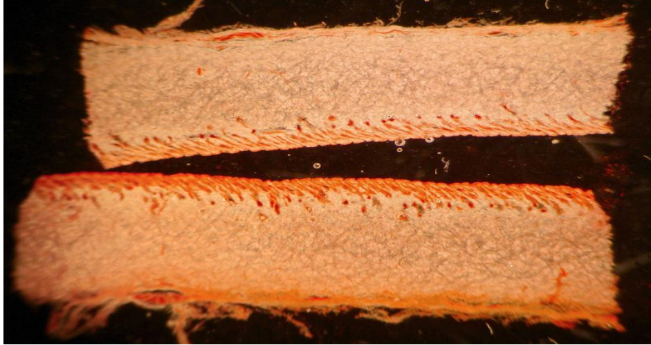
Fig.3. Sample BTR1 test on top and BCR-1 control on bottom showing full cross-section stained with Sudan IV to reveal fats. More intensely colored control indicates a higher residual fat content.
