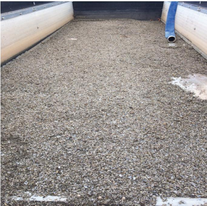
*Figure 1: Zebra mussels collected from the open recirculating cooling water system via strainers located upstream of the CCW and LRVP Plate and Frame Heat Exchangers while on the 12.5% bleach program. The program was supposed to prevent these mussels from even getting into the system in the first place.*
