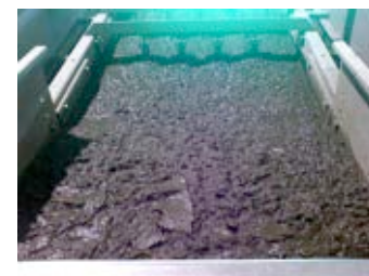
Extracted sludge on the sludge table depicts an improved sludge quality.
