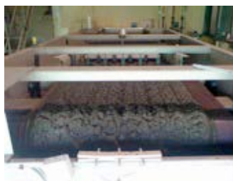
Extracted sludge on the sludge table depicts an improved sludge quality.
