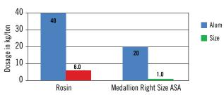
**Results:** Able to run with just 1 kg/ton Medallion RS160 and 20 kg/ton alum with sizing tests superior to rosin-based system. Medallion Right Size offers savings of US\$100,000/year, giving the mill the opportunity to develop new paper grades not possible with rosin sizing. In addition, we saw:
