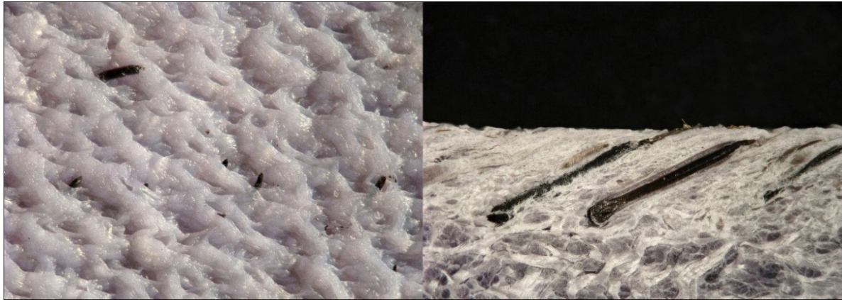
Fig. 7. Left optical photograph of wet blue with fine hairs. Right cross section of the wet blue showing intact hairs.
